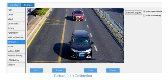
2) Click "Play" and when the vehicle plate comes to the bottom of the image, click "Pause". Adjust the size and position of the "Near" box to make it the same width as that of the plate.
